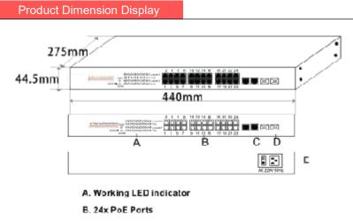
C/D. 2 Gigabit TP/SFP Combo Uplink Ports
