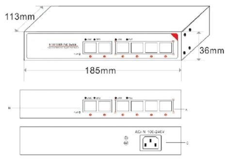
A. PoE Power Supply Ports B. Uplink Ports C. AC/IN 100-240V Input
